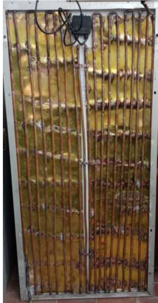
Fig. (1): Thermal heat exchanger at the back of the PV system
