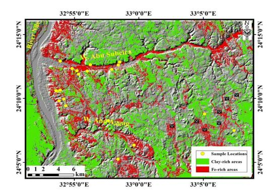
**Fig. 10:** The distribution map of the clay- and iron rich localities drapped over the hillshade map of the study area. This map is derived from the remote sensing data and verified by the field and stratigraphic studies. Note: the presence of the iron working quarries (black boxes) around wadi Abu Aggag at the extracted iron rich areas.
