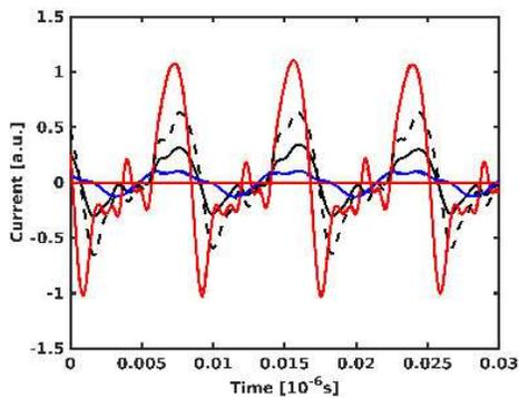
**Fig. 9.** The current passing through the discharge for different plasma simulation cases shown in Fig. 3.
