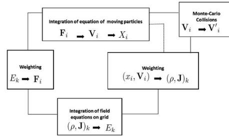
**Fig (2):** A schematic flow chart of PIC modules. The dashed lines are to short cut Monte-Carlo calculations for collisionless plasma.
