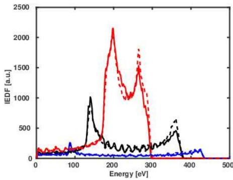
**Fig. 5.** The ion energy distribution function at the left electrode for different plasma simulation cases shown in Fig. 3.
