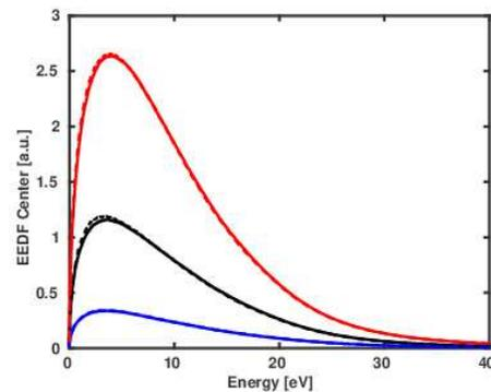
**Fig.7.** The electron energy distribution function at the center of the discharge for different plasma simulation cases shown in Fig. 3.
