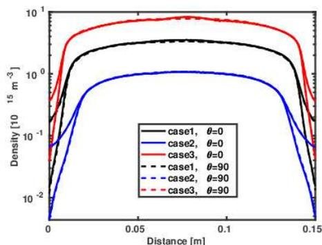
Fig. 3. The plasma density between the two electrodes.
