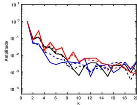
**Fig. 10.** The Fourier component of the current passing through the discharge for different plasma simulation cases shown in Fig. 3.
