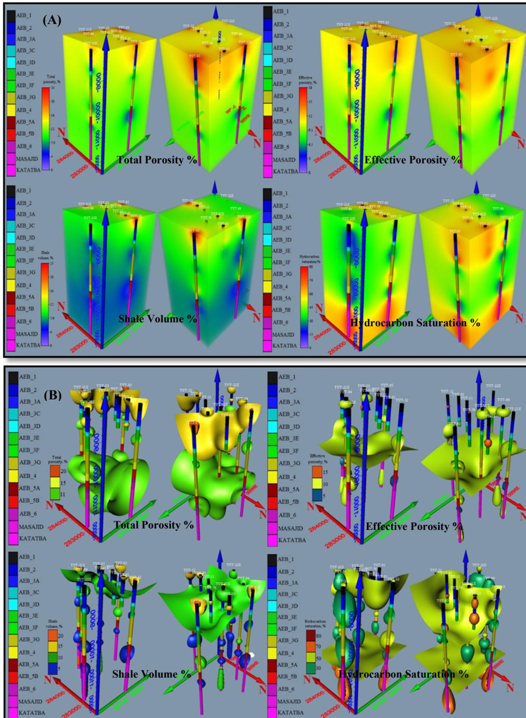
Fig. 6: Petrophysical parameters in 3D volume render (A) and isosurface (B) of TUT wells.
