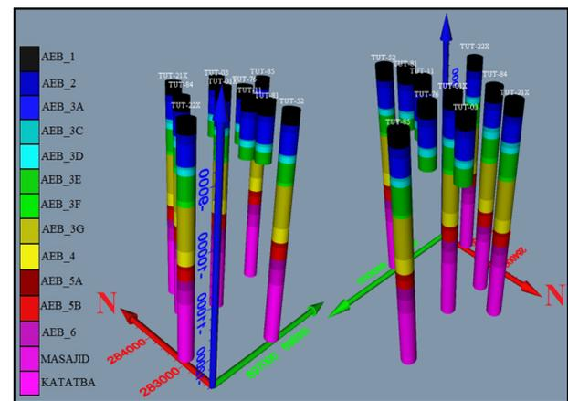
**Fig. 3: GIS 3D model of distribution wells in the study area of Alam El Bueib and Khatatba Formations.**
