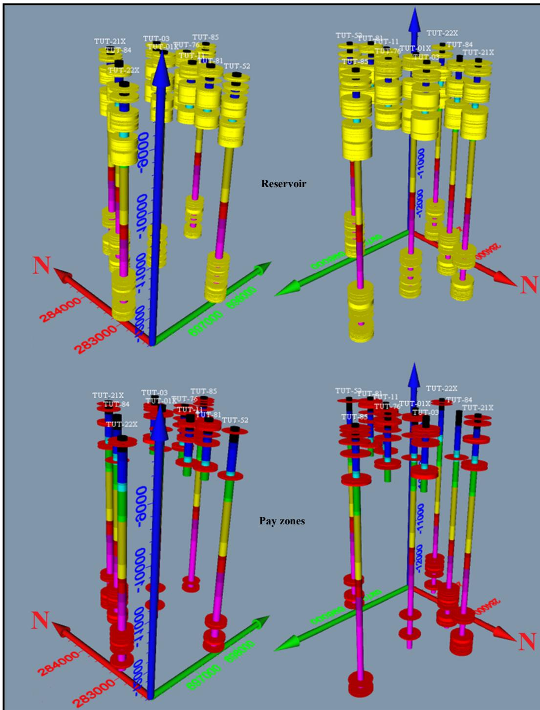
Fig. 7: 3D models of the reservoirs (up) and pay zones (down) of TUT wells.
