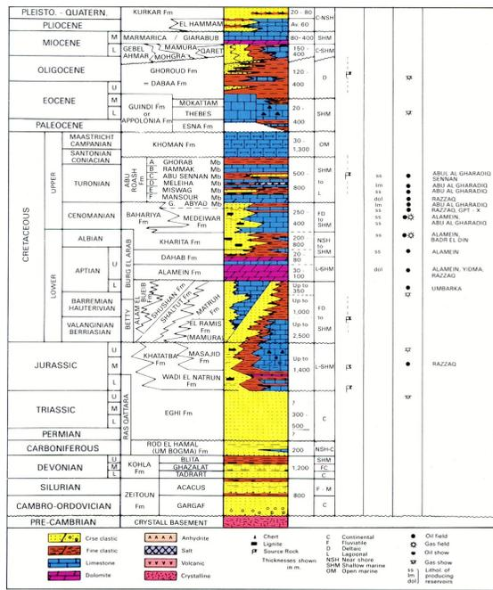
**Fig. 2: Litho-stratigraphic section in the northern Western Desert (Schlumberger, 1984 and 1995).**
