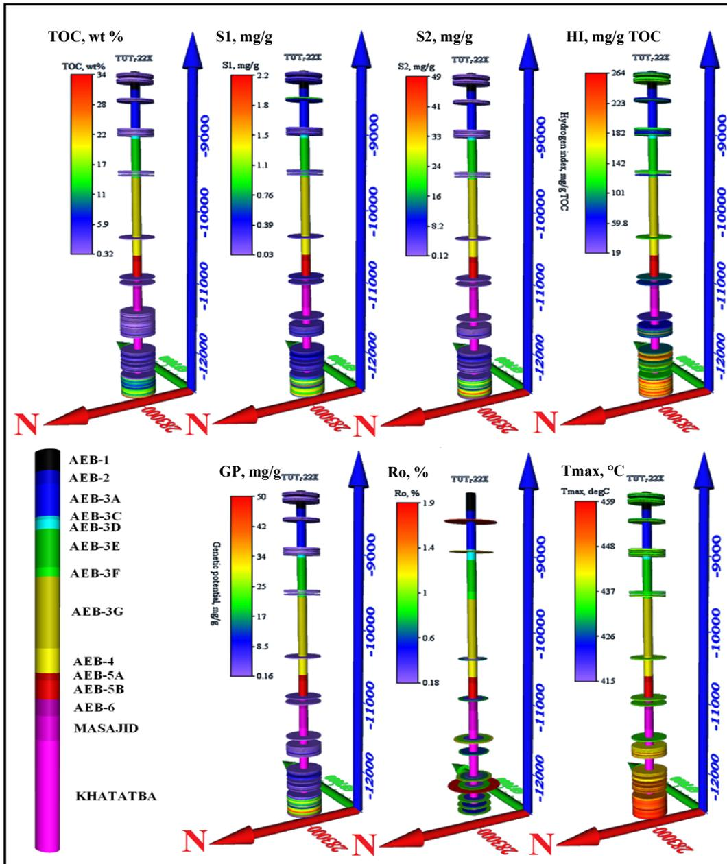
Fig. 4: 3D geochemical parameters for TUT-22X well.
