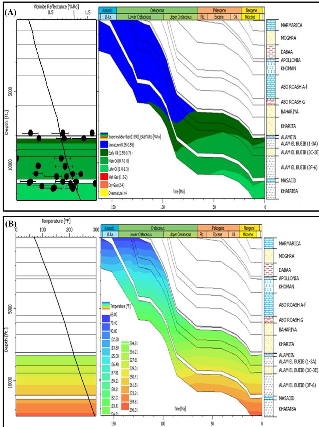
Fig. 5: Diagram discriminating maturity levels (A) and thermal burial history (B) in TUT-22X well.
